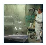
ProTegrity<sup>™</sup> is the Saratoga Spa® rigidizing system, replacing the previous 40lb foam system. ProTegrity<sup>™</sup>, according to Anthony Brennan, Saratoga Spas COO, "raises the rigidizing strength to 60 lbs, for a 50% increase."
