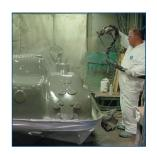
ProTegrity<sup>™</sup> is the Saratoga Spa® rigidizing system, replacing the previous 40lb foam system. ProTegrity<sup>™</sup>, according to Anthony Brennan, Saratoga Spas COO, "raises the rigidizing strength to 60 lbs, for a 50% increase."
