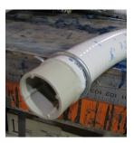
Saratoga Spa® Co. uses a Unique Design in plumbing its product. There is a three step process that the majority of the Saratoga Spa Models use; Barb-Glue-Clamp. Saratoga first glues the pipe and fitting, and then using a specially designed air pressure tool, it presses the plumbing fitting into the flex hose. This tool is calibrated to make sure that the fitting seats properly every time into the flex hose. This tool helps to eliminate someone manually having to push the fitting into the
